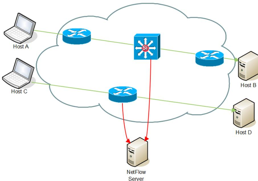
Figure above shows an example of communication when we want to monitor communication that is not passing through the central router. It is necessary to configure the NetFlow export on network devices on which that communication is passing through.
