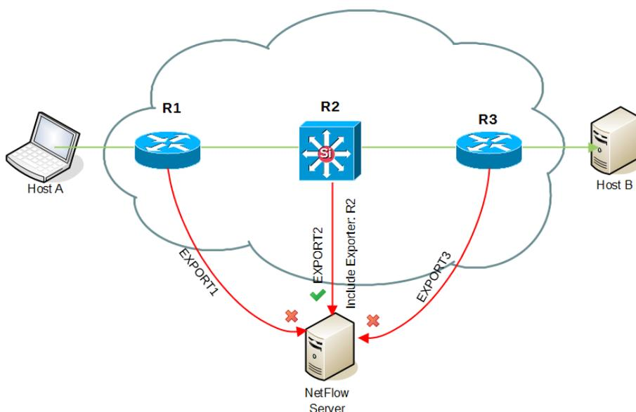
In our example above, flow that passes and is exported by three routers (R1, R2 and R3) will be taken into account and processed only from central router (R2) since Traffic Pattern includes its IP address in Exporter filter.
