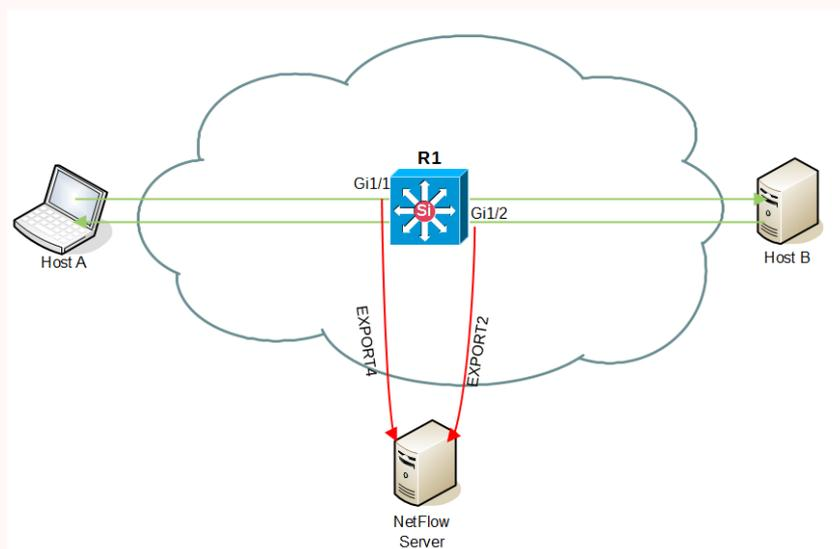
In Flexible NetFlow, *Input* and *Output* do the same as *Ingress* and *Egress* in Traditional NetFlow.
