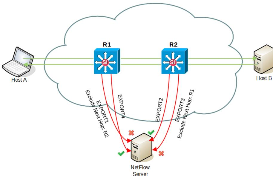
The solution is to exclude R2 as Next Hop IP address. This will simply skip all the flows passing from router R1 to R2. Flows will be then matched and processed only by router R2. The same applies for flows from Host B to Host A - excluding R1 as Next Hop will skip flows from R2 to R1.
