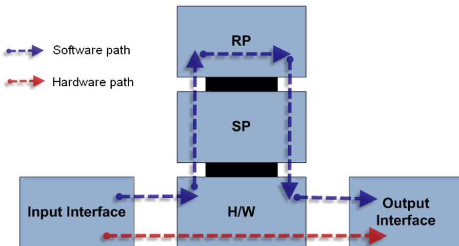
Figure above shows the concept of two paths for NetFlow packets, the hardware (red) and software (blue) paths and the configuration for each path. Normally on Cisco Catalyst 6500 Series Switch both hardware and software based NetFlow is configured.
