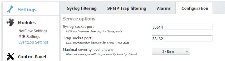
By default, syslog messages are exported from the devices to port 514, while NetVizura listens on the port 33514 in Linux systems and on the port 514 in Windows systems. If you use Linux systems, you need to (1) redirect syslog messages to the 33514 on NetVizura server, (2) export syslog messages to 33514 from device, or (3) change NetVizura EventLog configuration. Same applies to trap socket port.
