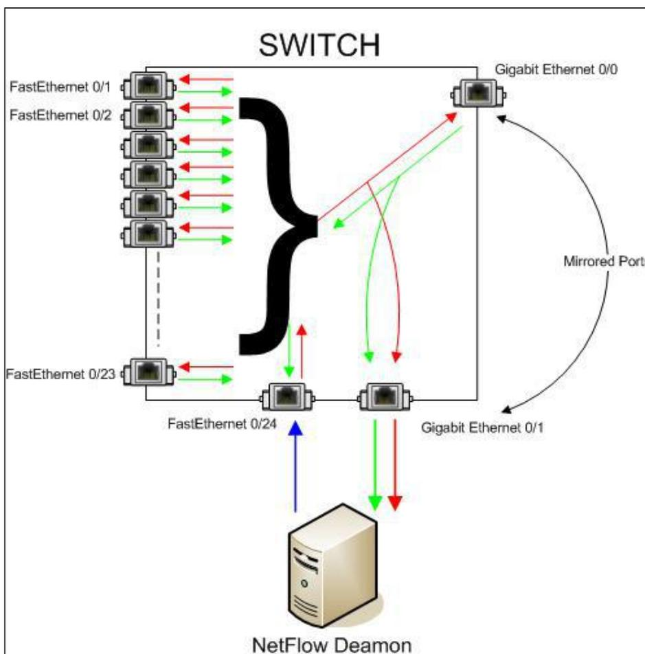
Figures above show the redirection of traffic (**port mirroring**) to the server on which the NetFlow Daemon Server is started. When the port mirroring is started on a switch, interface to whom all traffic is directed to becomes useless for normal device communication. It only passes all of its traffic (In and Out) from port mirroring interface.
