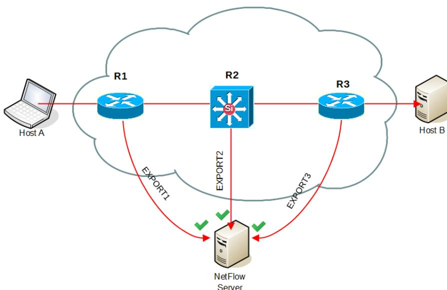
When automatic deduplication is disabled, a flow traveling from Host A to B and passes via multiple exporters, NetFlow Server will receive same flow from R1, R2 and R3 so flow will be processed three times.
