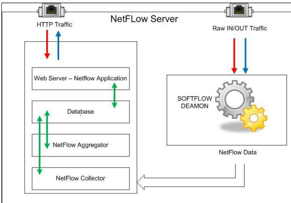
Now, it is possible to start the NetFlow probe on the NetFlow Daemon Server. One of these applications is the SoftFlowd that has the possibility of exporting NetFlow traffic locally (127.0.0.1) to the UDP port on the same server or to a UDP port on a remote server.
