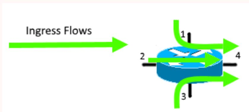
You should configure interfaces on a single device to collect flows in only one direction (either *Ingress* or *Egress*), so that flows traveling from one host to another and vice versa are collected only once.
